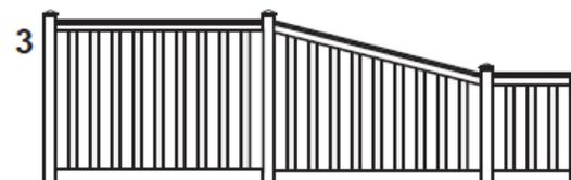
**3 TRANSITION:** A fence can be transitioned easily to a different height. Horizontal post spacing will need to be reduced and top rails will need to be miter-cut. Pickets will require cutting.
